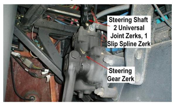
There are **THREE** Zerk fittings on the steering shaft and slip spline. **TWO** Zerks are on the two universal joints and **ONE** Zerk is on the slip spline shaft.
