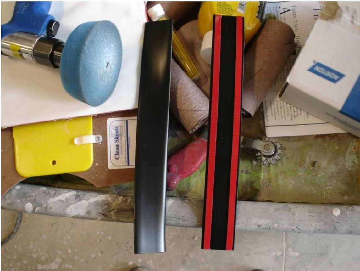
The two red protective strips are removed from the trim leaving an adhesive strip on the back which will stick the trim to the sidewall. The sealer filled sidewall cut is then straddled by the above trim strip.
