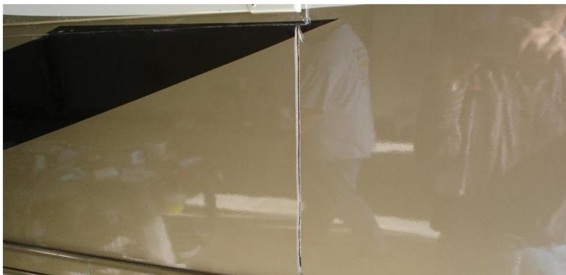
The above picture was taken after L.D. (tech) made the two relief fiberglass cuts under both ends of the slide. After the cuts were made he taped both sides of the cuts leaving the saw cut open. The open cuts were filled with filler which would stay pliable after it had cured. The tape was removed and the side wall was cleaned. Cleaning the sidewall provides a good surface for attaching the bridging strips to the wall.
