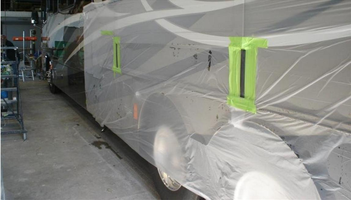
Below is the area of the driver's bedroom sidewall which cracked and repaired by L.D.
