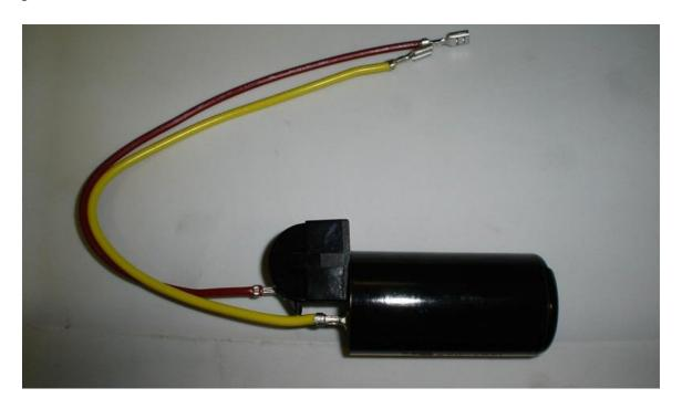
The small black bump attached to the red wire is the PTCR device. The PTRC device is itself attached to the start capacitor with a quick connect fastener. The yellow wire completes the kit.
