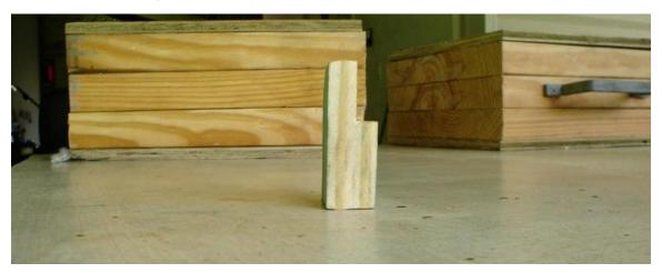
My, Low Tech Modification, three blocks of pressure treated wood cut in this shape. This shape allows mounting into the upper door channel. I decided on installing three blocks, left, right and center just for security. I cannot really supply any measurements because on my coach each block length was different. Left to right each of the blocks got shorter not by much but still they were each shorter. It probably has something to do with 3/16 ".
