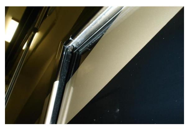
this compression the two "C" channels are pushed apart. When TMH installs the door the two "C" channels are tight but after dozens of open and close operations the aluminum wears just enough to allow the channels to push apart and unhinge.
