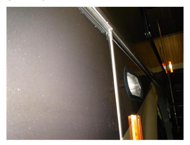
As seen in the above picture, this end of the hinge was not as bad as the left end however I do not think it would have been long before there would have been damage. I would never have been able to catch the door during opening or closing if the channels had become unhinged.
