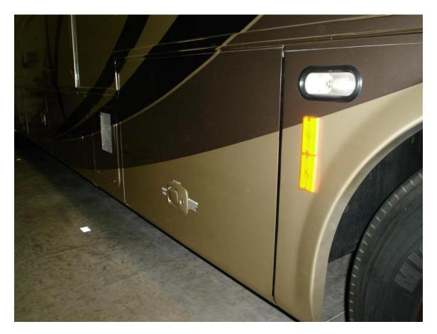
You can see the small 3/16 inch gap in the upper left top corner of the door. I see no way to correct this assembly error after the fact I'll just live with it. This modification took three hours of my time I used a few inches of pressure treated wood (3/4" x 1 1/2" x 2 1/2") for the blocks. A few dabs of black silicone and few wisps of black spray paint so the wood would blend in with the surrounding black painted metal.
