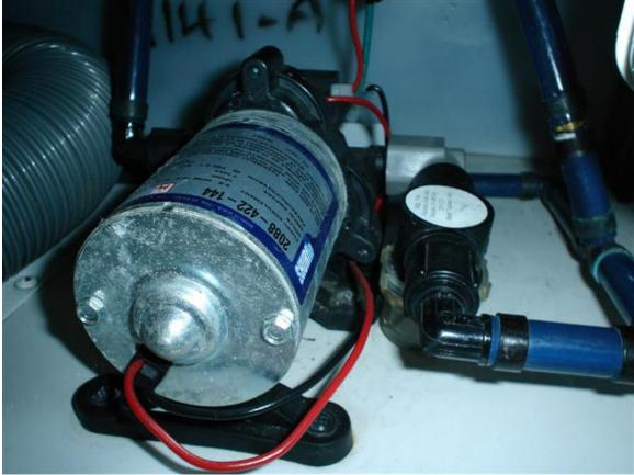
If the first step did not correct the problem, we move on to step two. This next step is to make sure that the battery is sending +12V to the fuse. My fuse panel is under the Norcold refrigerator, the fuse is labeled "Water Pump". Test the voltage on both sides of the fuse with either an electrical meter or a test lamp. Now make sure that same +12 volts is getting to the latching controller at the +12V red wire.
