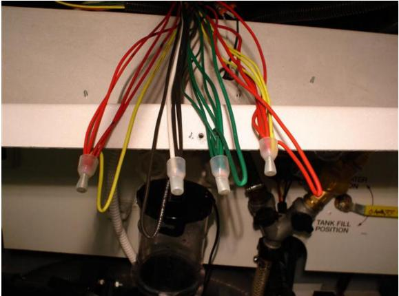
I folded back the four water pump controller wires the Yellow (SW) wire (on the left) is spliced to four red wires. The Black (Gnd or Ground) wire is spliced to four other black wires and one white wire. The Green wire (load) is spliced to five other green wires. And the Red (+12V) wire is spliced to three other red wires and three yellow wires.
