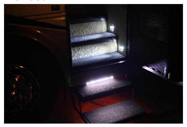
Now when the door is opened, all step LED's turn ON. The area around the steps is well lighted. Now the top surface of the outside and inside steps is illuminated and not just the underside of the outside steps and the right half of the inside steps.
