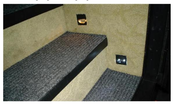
Both fixtures below have been modified with the Super Bright LED's. Both outside steps had previously been modified by adding LED strip lighting to illuminate the top of the step treads.
