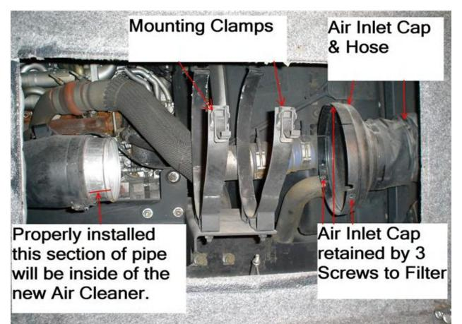
7. Now that you have the old filter out of the way. Remove the clamp from the air inlet cap and hose. You may need to be gentle, use something to loosen the hose away from the cap. Once the cap is loose, remove it from the hose.
