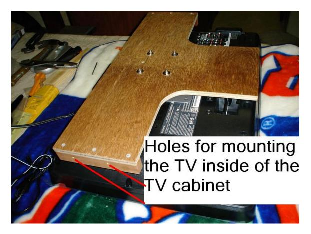
The bottom edge of the plywood "T" mount in the picture below rests on top of the felt strip glued to the top of the remote control cabinet.
