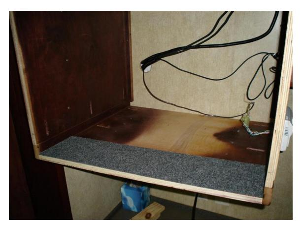
We had decided to make and install a cherry hardwood shelf for the TV to sit on and also provide a small shelf for the remote controls when not in use. As you can see in the below picture we did not remove the top felt padded piece of wood Tiffin had installed to prevent the OEM TV from moving back into the cabinet space. This piece of wood is secured by screws through the outside walls of the cabinet, removing this piece of wood would have been destructive to the cabinet.
