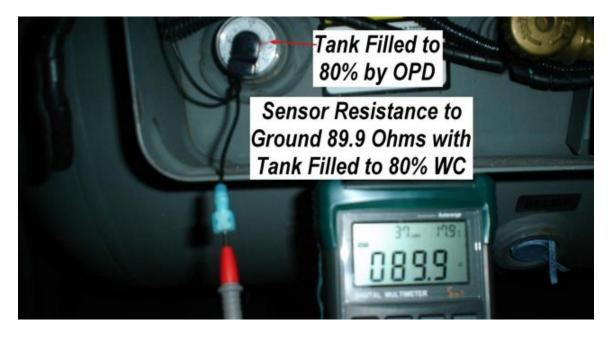
The tank is full at 80% (WC) capacity the tank sensor resistance to ground was measured at 89.9 Ohms, as shown on the meter above.
