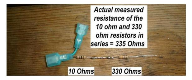
The two resistors soldered in series ACTUALLY MEASURE 335 ohms. The green wire with the 1/4 inch male and female connectors when mated with connectors installed on the LP tank sensor wire and the SeeLevel monitor wire form a parallel circuit with the 335 ohm resistor connected to ground. The finished modification has the LP tank sensor and SeeLevel system resistance wired in parallel with the 335 ohm resistor tied to ground.
