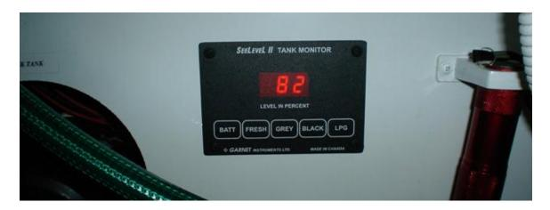
In this case the tank sensor is reading around 56% while the wet bay display is reading 82%, the display was last calibrated during the summer while temperatures were higher.
