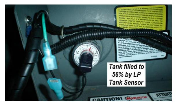
After a little planning and dragging out my rusty electronic formulas I figured a way to obtain a displayed tank fill value closer to reality. If 89.9 ohms displays 100% on the SeeLevel monitor what do I need to do for the display to show what is really in the LP tank. When the tank is full at 80% WC I want the display to read 80% or close to 80%.
