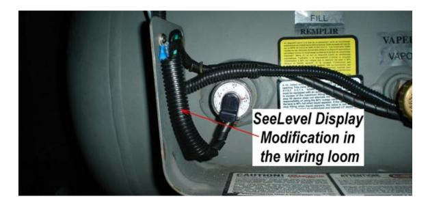
After the parallel resistor modification when the tank is filled to 80% which is actually FULL instead of the SeeLevel system displaying 100% both displays will now display a percent level closer to the actual LP tank fill, even with the 2% SeeLevel display error the filled tank is displaying 81%.
