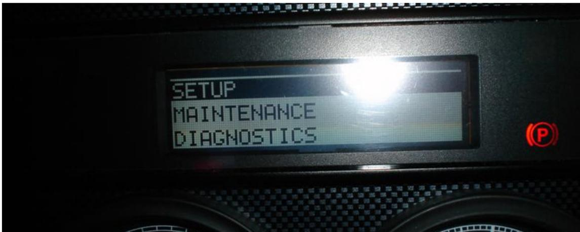
When you see the above screen, **DOWN TOGGLE TWO TIMES AND RELEASE** the button. Then **RIGHT TOGGLE AND RELEASE** the button. After the menu updates you see the following menu.
