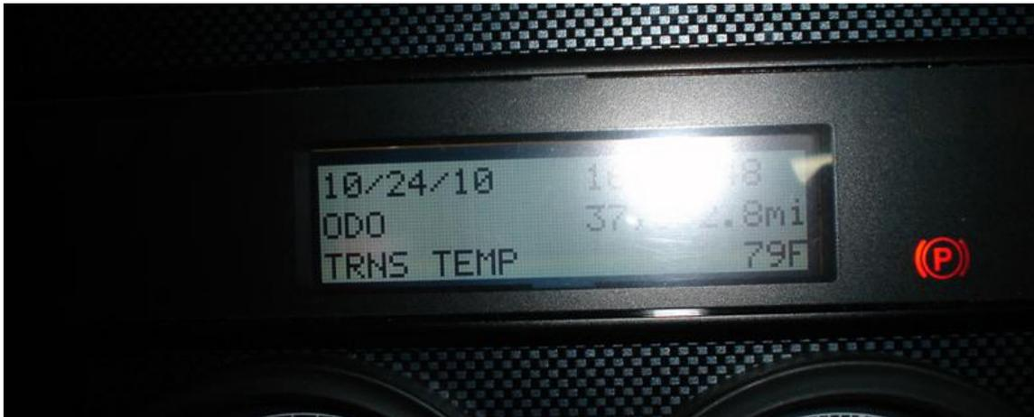
Once your display looks like the above or else your three favorites. **RIGHT TOGGLE AND HOLD** the menu toggle switch until the next screen is displayed. It will take about **5 SECONDS** to display the Setup, Maintenance, and Diagnostics Screen, like seen below.
