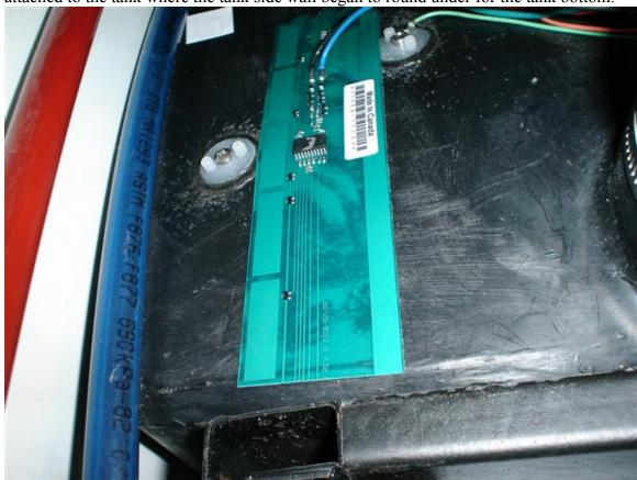
As you can see, I did not need to shield or remove any steel for this install. The end of the sensor is about 3/4 of an inch from the metal frame.
