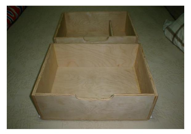
The bottom drawer has a small divider which will keep a few black tank chemicals separated from the blow dryer and curling irons. The top drawer will hold the necessary back up supply of toilet paper and any other water closet necessities. I purchased the 1/2 inch plywood at Lowe's for this project. Lowe' did not stock the 12 inch drawer glides, I found them at Home Depot for \$ 4.99 each.
