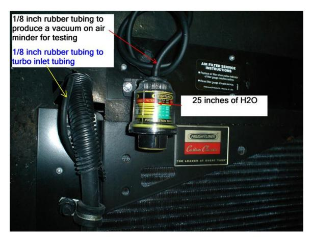
By pushing up on the bottom of the indicator you can reset the diaphragm to the bottom on the indicator. The bottom is usually around 6 or 7 inches of H2O.
