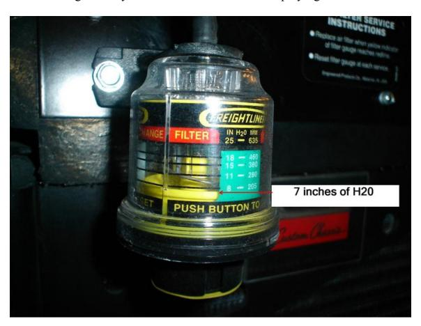
This coach is our third Freightliner chassis, we have had one each Caterpillar, Cummins and now Mercedes Benz powered coaches. The air restriction indicator on the Cummins ISB started at 11 to 12 inches of H2O. The Caterpillar 3126E started around 8 inches and the Mercedes Benz
