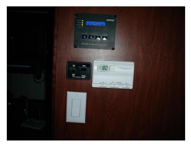
My second project was to install the See Level 409 tank monitoring system, one monitor was installed in the wetbay and a second monitor was installed in the hallway on this same wall as the Xantrex remote control panel. The wiring for the tank monitor was routed through the same area as I had for the Xantrex remote.
