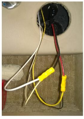
with split loom before being routed along the right chassis frame to the rear of the fuel tank where both driver side and passenger side LED light strings are secured inside of the lower coach frames.
