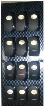
clear tubing. Seen below when the Assist Handle switch is turned ON (Red LED illuminated). The inside and outside assist handles are illuminated along with the two NEW strings of LED's under coach lights.
