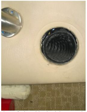
piece of wire with a hook in one end was inserted thru the hole made by the wood dowel to capture a pair of 16 gauge zip wires. The zip wires are covered and protected by a black <sup>1</sup>/<sub>4</sub>" split loom, the loom was installed over the complete length of wiring to both sets of LED's.
