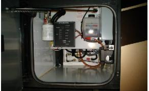
Now when it is time for the annual fuel filter changing, the shut off valves are turned off then the filter is unscrewed after first placing a catch basin under the filter in the event I get messy while removing the old filter. The new fuel filter is prefilled thru the filters small outside holes while keeping the filters center hole plugged. Filling the fuel filter this way the prefilled fuel passes thru the new filter before it reaches the Aqua-Hot's fuel solenoid.
