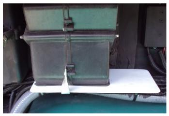
The photo on the left was taken while testing the idea, a piece of 1/8" aluminum stock cut to the normal license tag size of 6" x 12" was used. Following months of testing I decided to make the vent cover a semi-permanent modification. Rather than use the metal tag plate I opted to cut up an old plastic tag as seen below.
