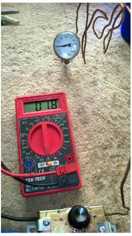
In both above photos a thermometer was tie-wrapped to the thermostats thermocouple bulb. To lower the thermocouple's temperature for testing the thermocouple was immersed in a mug of ice and water which lowered the thermocouple's temperature down to the mid 20° range.
