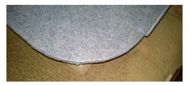
After the rounded corner had been cut, a belt sander was used to smooth the plywood, the smooth plywood surface allowed the felt to be re-glued to the plywood. A heavy duty spray adhesive was used to glue the felt back down after the glue had dried excess felt was trimmed off with a razor knife leaving a smooth surface.
