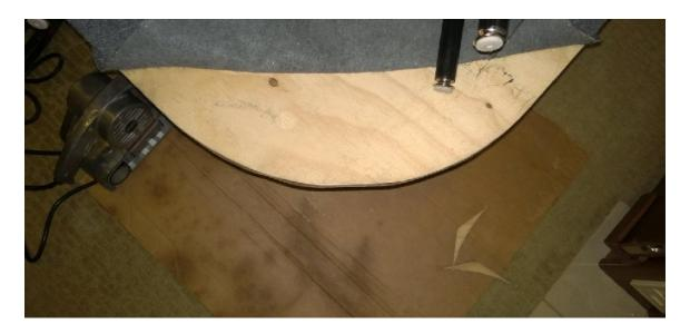
A 12 inch set of dividers was used to scribe a 12 inch ¼ circle, the line was used as a guide for cutting the plywood with a Saber saw.
