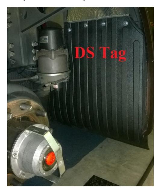
The 30 inch width of both rear skirts completely blocks the area between the coach sidewall and the chassis frame.
