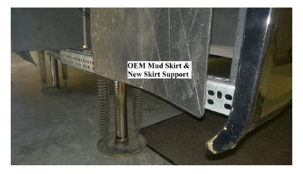
Construction of D/S and P/S front skirts and installation are the same.
