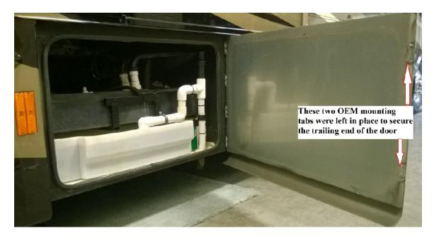
As seen above the TWO left side mounting tabs were not removed as those tabs are used with two long screws to secure the door in the closed position.
