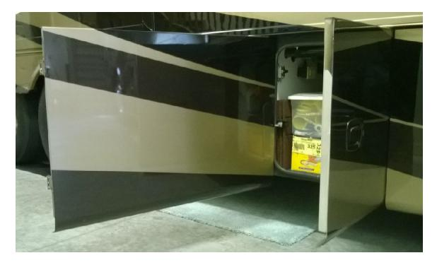
As an added benefit if additional heated storage were needed there are several cubic feet of space on top of both black and gray tanks.
