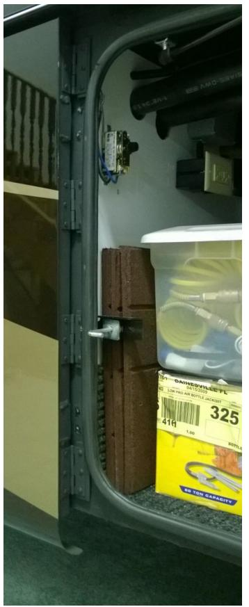
The photo on the left shows the installation of the four hinges to the wall of the coach basement. Attachment of the hinges to the coach was done using  $\# 10 \ge 32 \ge 10^{\circ}$ 1" stainless steel screws and nuts.
