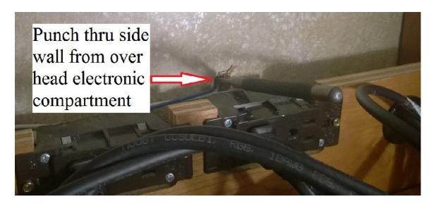
As seen above a pin punch was driven thru the hole drilled in the wall for the awning wiring. Care was taken making sure the punch did not damage the door awning wiring. Tiffin used some form of hard rubber to seal the hole drilled thru the wall. Every time the punch was removed the hole would attempt to re-seal itself.
