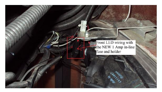
The above photo shows the installation of the fuse holder for the FRONT clearance lights, I also installed a label stating the name of the circuit the 1 Amp fuse is protecting.
