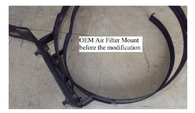
Comparing the above and below photos the  $\frac{1}{2}$ " bolts, lock washers and stud nuts push the air filter bracket straps forward about 1  $\frac{3}{4}$ " which almost centers the air filter between the closet wall and the rear cap fiberglass.
