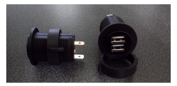
I ordered the chargers with what is called a Q (Quick) Nut, the threads inside the nut allow the nut to be slid over the threaded portion of the charger until the nut is tight against the dash then the Q nut is turned 90 ° to lock the nut
