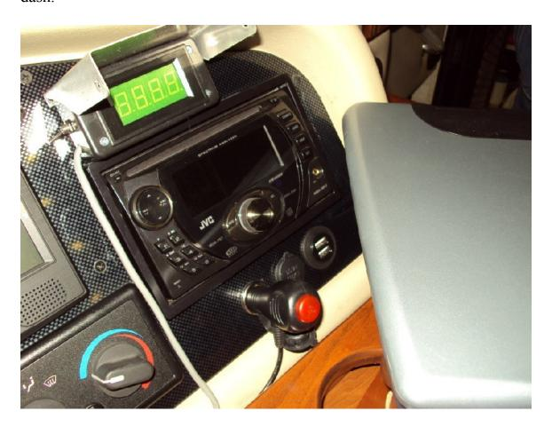
The two USB chargers add four new charging ports in the cockpit, I can also plug into the two above dash 12 VDC outlets, then plug in a 12 VDC to USB A male to Micro USB male cable OR plug in a USB A male to Mini USB male cable to recharge my cameras.
