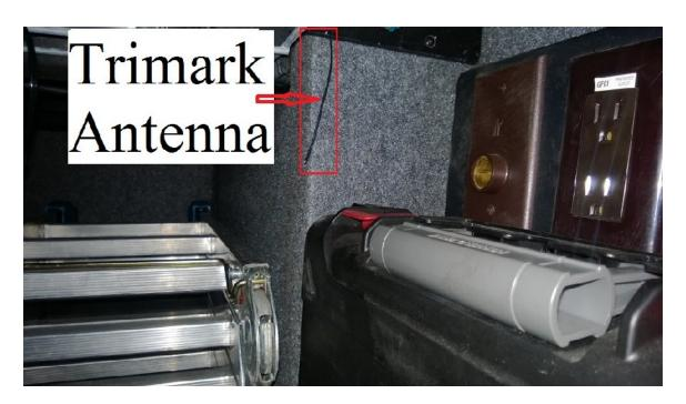
As seen in the above photo, the Trimark Keyless Entry antenna when fully extended is only about 6 to 7 inches in length.
