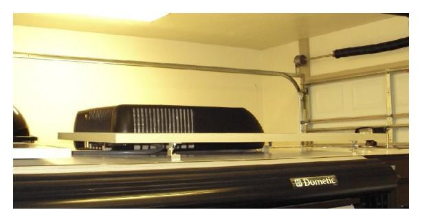
Black nylon zip ties were installed around the pivot brackets where the PVC electrical tubing passed by them to prevent the tubing from shifting around making marks on the roof and also making noise.
