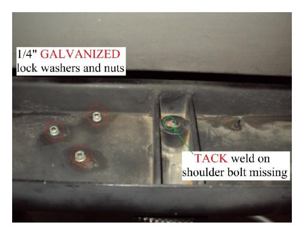
After everything was installed and tightened it is my hope this modification will prevent the loosening of the step motor bolts in the future, however time will determine if that is true.
