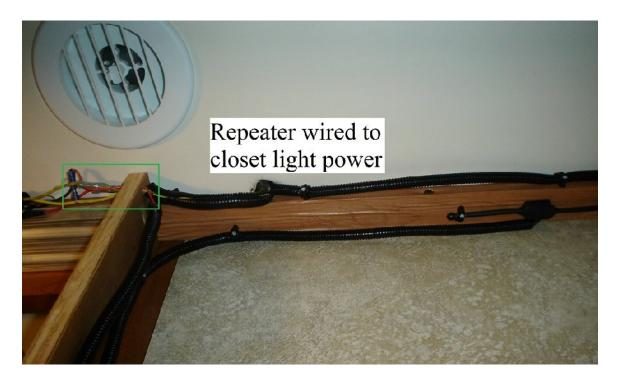
As seen above the power for the two closet lights can be seen in the above green square. The repeater circuit required a ground wire (12- VDC) to be tied into the mirror lighting circuit as Tiffin did not need or run a ground for the closet lighting.
