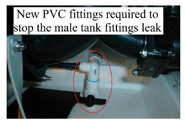
After the above fittings were installed a new 90  $^{\circ}$  adapter was installed along with the brass female hose connector and new easier to remove/install plug.
