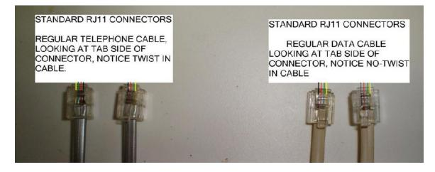
The PHONE cable connectors on the LEFT are standard four conductor RJ-11 connectors. The two connectors are mirror images of each other, the wires are reversed. The DATA cable connectors on the RIGHT are standard four conductor RJ-11 connectors however the cable ends match each other. **ONLY ONE DATA CABLE** is used when installing the PI-EMS unit. That DATA cable is installed between the EMS and the data switch or the display depending on a single display or a dual display.
