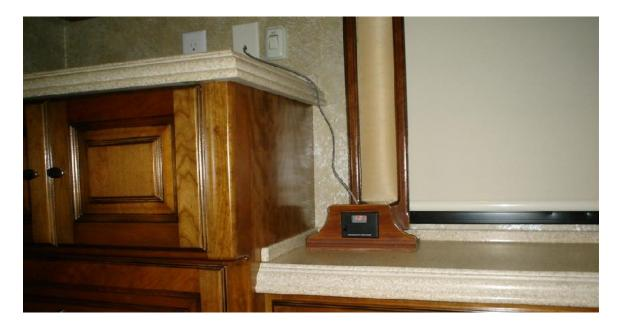
A display stand was built stained to match the woodwork in our coach the display can be inserted then the stand which may be placed almost anywhere in the coach. I find it very convenient to have the display located in the bedroom where it can be seen during the night to make sure shore power is operating and the coach is not running off the inverter.
