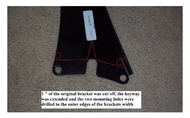
As noted above the width of the bracket became a problem after the bracket was shortened. I do not think there will be any future problems as the two bolts securing the bracket to the transmission housing tightened completely. The bracket was installed then the exhaust pipe was mated to the turbo flange in the flowing photo.
