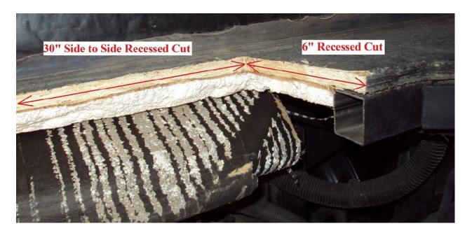
The fiber paper glued to the Styrofoam under the OSB floor was pulled back before cutting the steel tubing and OSB flooring to be used later to protect the finished floor modification.
