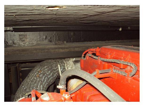
After removing the exhaust transverse pipe to allow better access to the section of floor to be modified while at the same time allowing me to test the bellows portion in this section of pipe checking for any hidden exhaust leaks.
