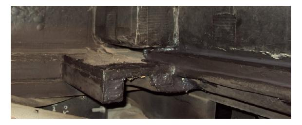
After a much need rest also to allow the silicone to cure Part B will take shape when the bellow section of the exhaust system is reinstalled. The new heat shield will then take its place.
