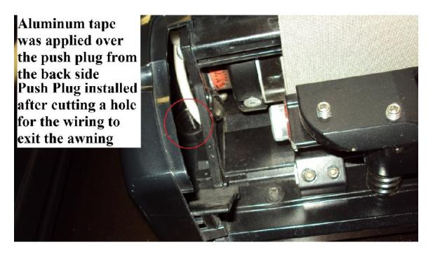
Two PLASTIC Push Plugs were purchased from Lowe's hardware section both plugs were pushed into the opening from the outside after which a piece of aluminum foil tape was applied over the plug to seal it in place. The left end plug required cutting a side opening in the plug to allow the awning control wiring to pass thru.
