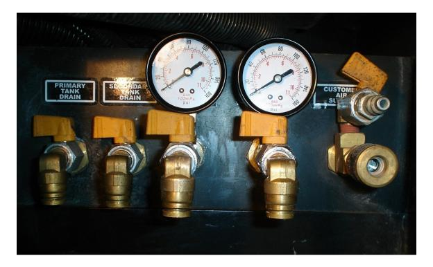
After experimenting with 40 PSI, 35 PSI and 30 PSI air pressure settings in the tag axle air bags, 30 PSI in the Tag Axle Air Bags was found to be the best weight balance for this coach. This pressure allows the front axle to carry 14,970 lbs., the drive axle to carry 20,130 lbs. and the tag axle to carry 4,600 lbs., the TOTAL COACH WEIGHT is 39,700 lbs.
