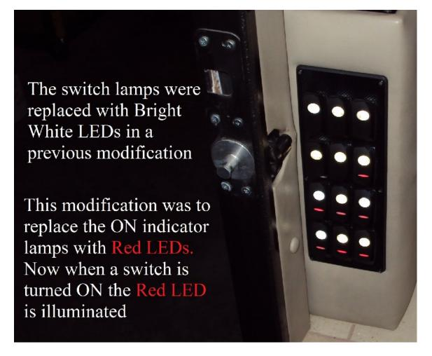
This is a simple low cost but time consuming project. I like the way the finished panel looks the only part I would have done different would be to use a lower light output LED in place of the Bright White LED in the switch logo light. However this amount of illumination serves great to light up the step well.
