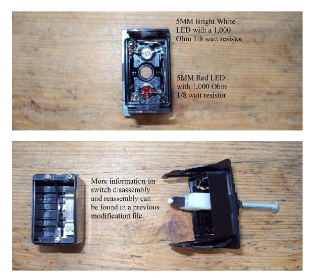
As shown in the first photo I decided to use 5MM LEDs for one simple reason they fit the hole in the switch vacated by the incandescent lamp.
