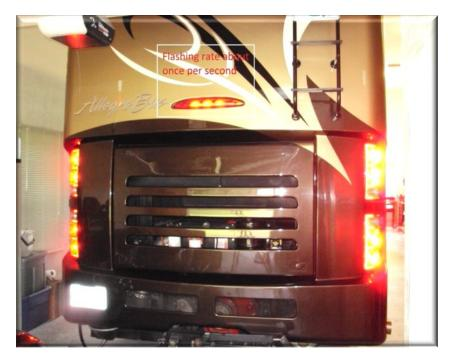
As noted in the photo, the third brake light flashes about once per second but ONLY while the service brake is being depressed.
