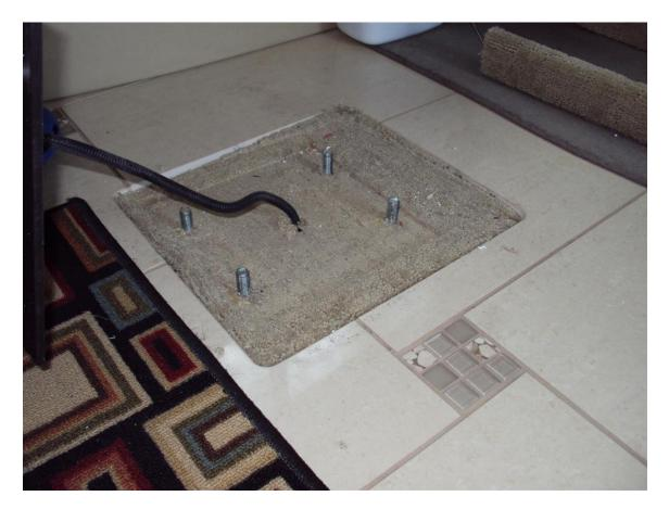
The bolt pattern on the pilot seat is 4 1/2 inches wide by 7 3/8 inches in length. Four 1/2 inch couplers were screwed onto the four 1/2 studs welded to the chassis frame in the Tiffin welding shop. After the seat mount was set down over the four couplers four 1/2 inch bolts one inch in length were screwed into the couplers. This modification raised the pilot seat about 2 inches higher then the OEM installation.
