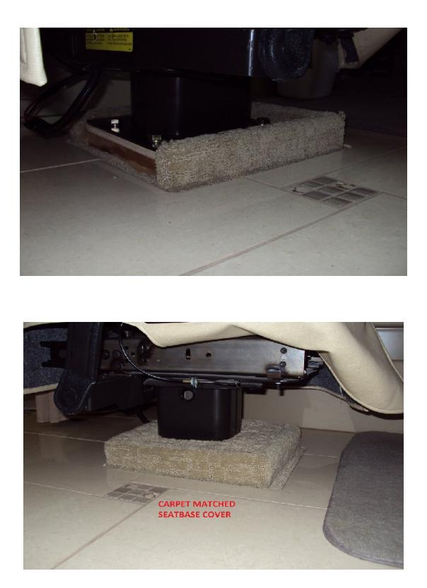
The Pilot seat mount revision cost was around \$ 60.00 as no 1/4" steel was needed and less hardware was needed to just raise the seat by 2 inches.
