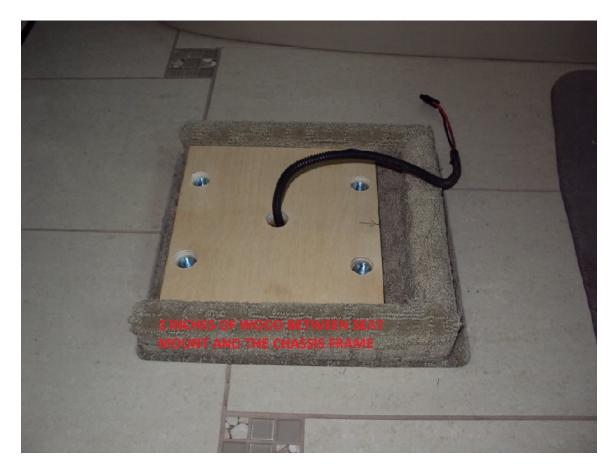
To provide a solid foundation between the seat mount and the chassis frame as piece of 2 x 10 yellow pine was cut 9" x 9" x 1 1/2". To finish filling the gap a 1/2 " piece of plywood was cut the same dimensions as the pine. This wooden installation was performed on both Pilot and Co-Pilot seat mounts. After installing the seat mount, the bolts were installed and tightened until there was no gap between chassis frame and seat mount which was not solid wood.
