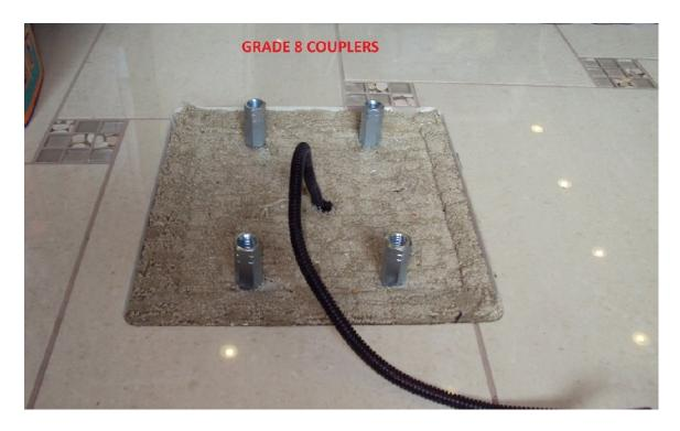
This modification was not what I would place in the easy and cheap modification category. Just the four grade 8 couplers FOR EACH SEAT cost \$ 50.00 along with the 1/4 inch steel plate, nuts, bolts and washers the modification cost for the Co-Pilot seat was around \$ 80.00. To allow Cathey to be more comfortable while we are traveling is PRICELESS.
