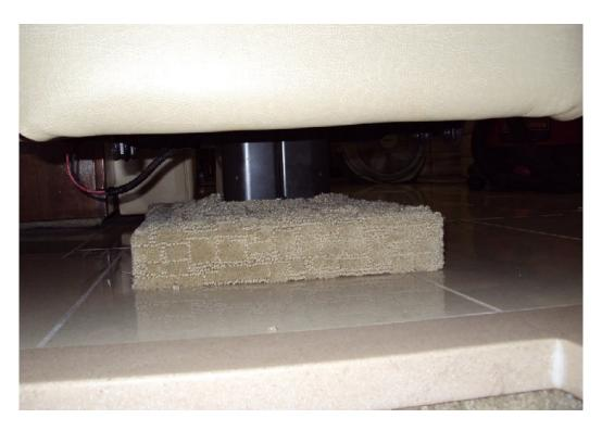
After everything was bolted and screwed in place, a piece of matching carpet was attached to a piece of wood which was used to close in the fourth side of the Tiffin installed seat base carpeted trim.
