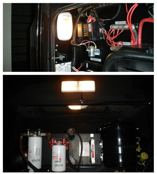
The nine original cargo lights draw 10 Amps, adding the three new lights drawing 5 Amps for a total cargo light power draw of 15 Amps on a 20 Amp "Cargo Lighting" circuit breaker located in the passenger side rear compartment.
