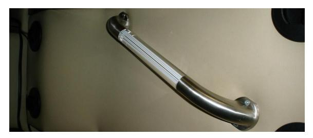
As seen in the two photos IMO the intent of the original black tape was to keep the lower metal bracket from being disconnected from the upper metal handle with the glued in glass rod from being separated DURING SHIPMENT. I think after making this modification the assist handle as it is now installed, is how the manufacturer intended the handle to ALWAYS look after installation.
