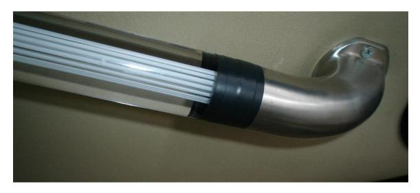
Yesterday after seeing the black tape had begun to unravel I decide to remove the handle after cleaning the residue from both the glass and metal then re-tape and reinstall the handle.
