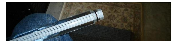
The "O" ring is a standard R14 1/8 inch thick ring. I decided to replace the "O" ring with a ring the same inside and outside diameter but was thicker 3/32 inch instead of the OEM 1/8 inch thickness. The ring was lubricated to allow the glass rod to be easier inserted into the metal end bracket.
