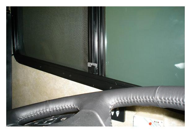
With the screen latch in this position when the window is powered open the screen opens with the window, also when the window is powered closed the screen and window are both closed at the same time. Just flip the latch up to disable the simultaneous window/screen function.
