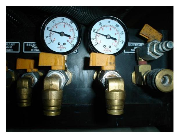
The driving test begins tomorrow we will be on the road for a few days. This permanent gauge setup should allow us to observe what the actual air pressure is in each side of the tag axle suspension. The gauges were installed into the PS and DS ping tank plumbing before the manual drain valves located in the DEF tank compartment.
