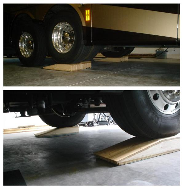
Each of the six ramps weighs approximately 20 pounds, driving up on the ramps allows the coach to be elevated five inches at the same time fully supporting the coach's weight without damaging the tires.
