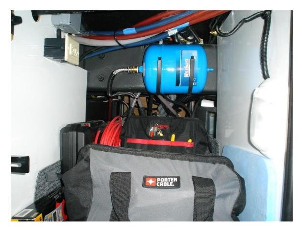
The gray ABS box located in the upper portion of the photo contains the Jenn-Air wiring running from the coach circuit breaker panel to the cook-top in the kitchen. The only additional components needed the black plastic box, a 20 Amp GFCI outlet, short piece of Romex cable, two Romex cable connectors, two self-tapping 5/8" drill screws and a short piece of 3/8 " wire loom to protect the Romex cable.
