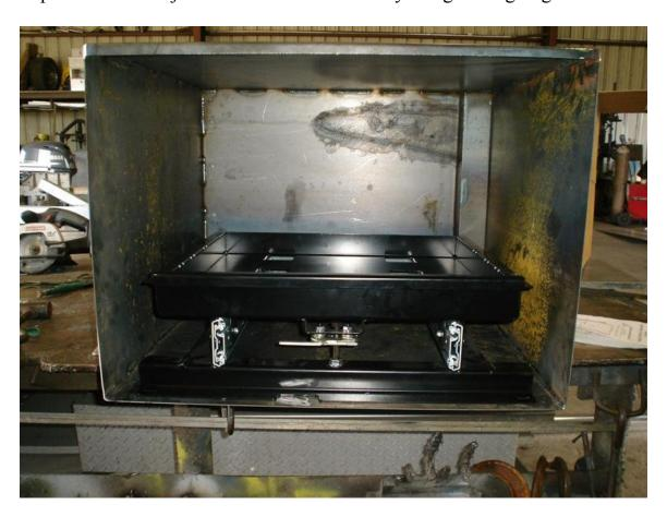
Today we picked up the new PS battery box. Now the fun really begins, we took time to dry install the box in order to mark where the bolt holes will be drilled to mount the new battery box to the chassis. We also marked and drilled holes for mounting the battery slide tray in the box once the battery
