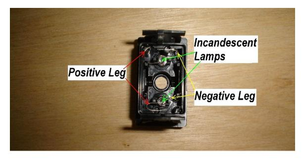
The upper lamp (switch lamp) is removed along with two plastic posts used to hold the lamp in place. The lower lamp is illuminated when the switch is turned ON. After the lamp has been removed the LED and resistor package are installed in the same location vacated by the incandescent lamp filament.
