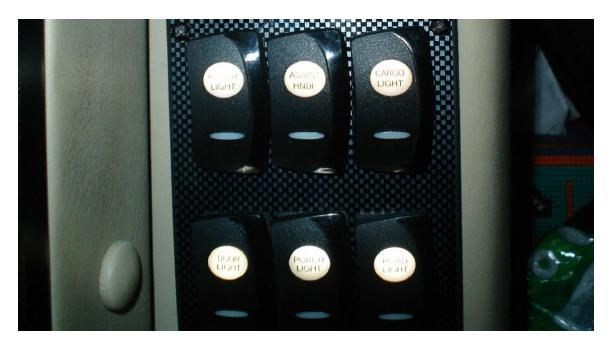
For less than \$ 20.00, 12 - 5mm White LEDs (Radio Shack # 276-0017) along with 12 - 1,000 ohm 1/8 watt resistors (Radio Shack # 271-004) were installed in the entry door switch panel.
