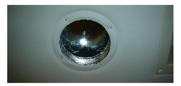
A razor knife was used to cut the white ceiling fabric along the pencil line. Then an air powered body saw with a fine tooth metal blade was used to cut the ceiling panel and its attached foam.
