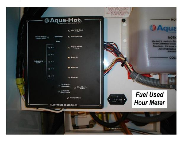
Now when I fill up with diesel fuel I can look at the Aqua-Hot Fuel Used Hour Meter. At the next fuel fill up I can use the hour meter to figure the actual hours the Aqua-Hot's Fuel Valve was open allowing me to figure the coach engines fuel usage even closer than I can now.
